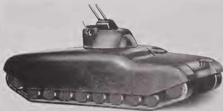
FIGURE 5. Model of IVI-D medium tank equipped with two 37-mm guns.
